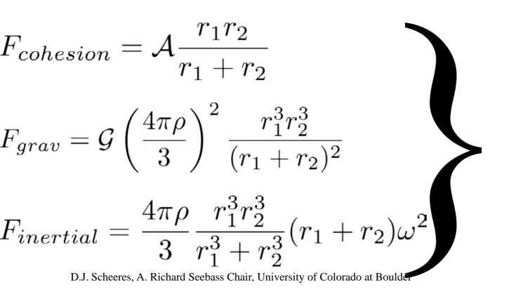
$$F_{cohesion} > F_{inertial} - F_{grav}$$
