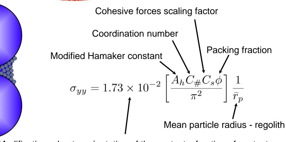
Modifications due to: orientation of the contacts, fraction of contacts in tension and magnitude distribution of cohesive forces.
