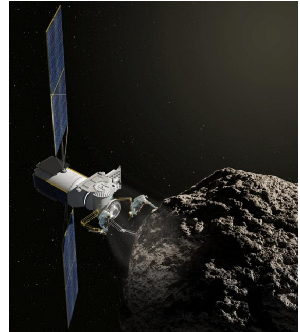
SEP-based excursion vehicle concept for human NEA mission (image credit: NASA/AMA, Inc.).
