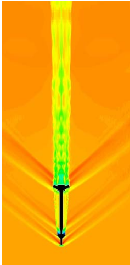
Figure 8. Calculated wave pattern for a conventional guided bomb at 1.4 kft/s
