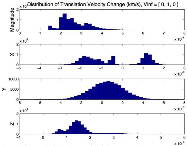
Figure 1: Histogram of delivered change in velocity to asteroid Golevka from a 1500 kg impactor striking the surface at 10 km/s with a 3-sigma targeting uncertainty of 25 meters (an accuracy of 0.1 asteroid radii).
