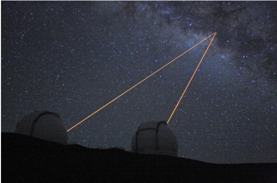
Figure 6. Adaptive optics is routinely employed in high resolution astronomy. The Keck telescopes at Mauna Kea uses adaptive optics to resolve the Sagittarius stars in the Milky Way galactic center. Reference beams such as these can be used to compensate for atmospheric disturbances while QBOLT system targets asteroids at 1-2 AU distances.[pic credit UCLA GCG]
