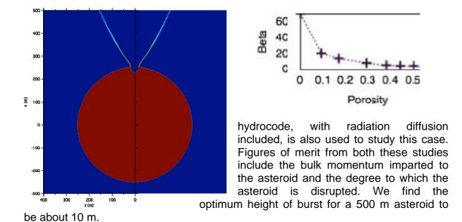
Figure 2. Left is a density plot at 14 seconds after a 600 kT burst at 5 m standoff distance from a 500 m diameter basalt sphere. Above is plotted the run of final axial velocity against standoff distance for three different burst yields.
