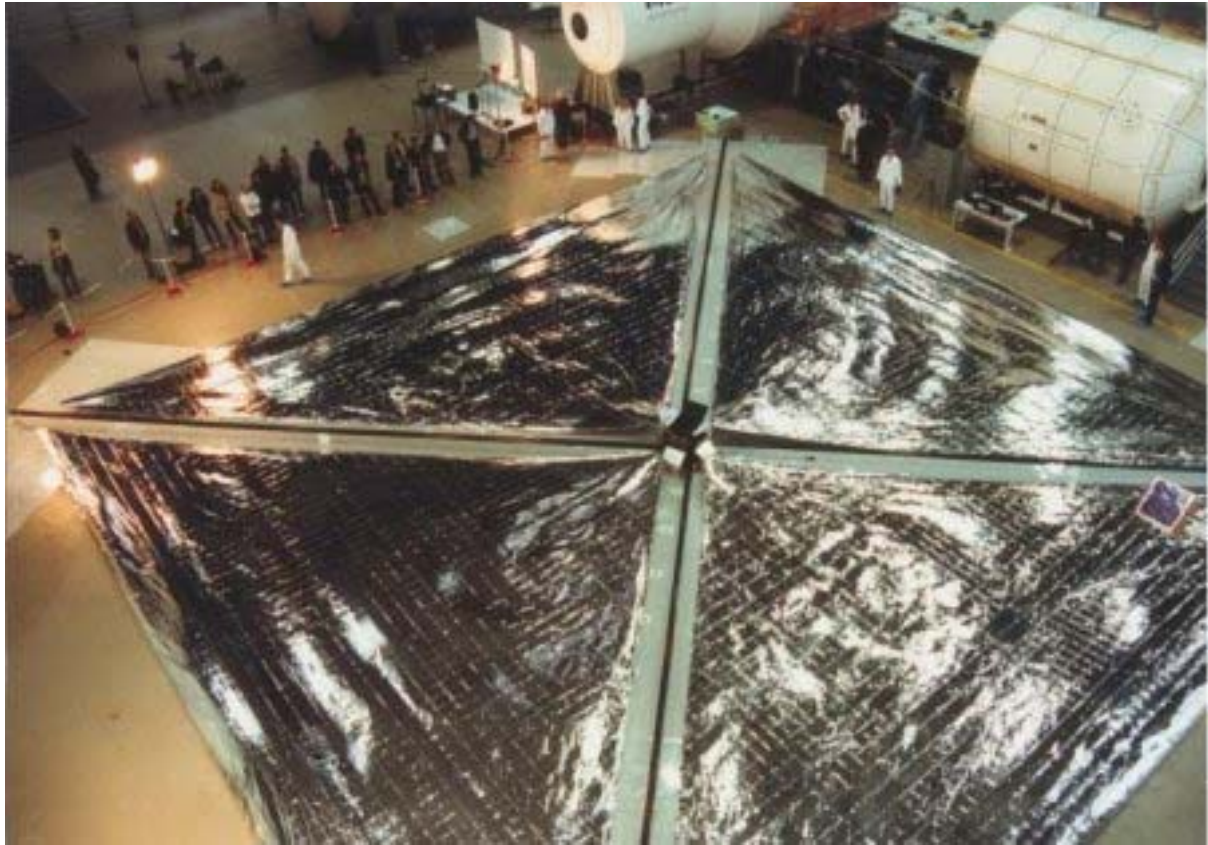
Figure 1 – Ground deployment test of a (20\text{ m})^2 sail at DLR Cologne, 1999
