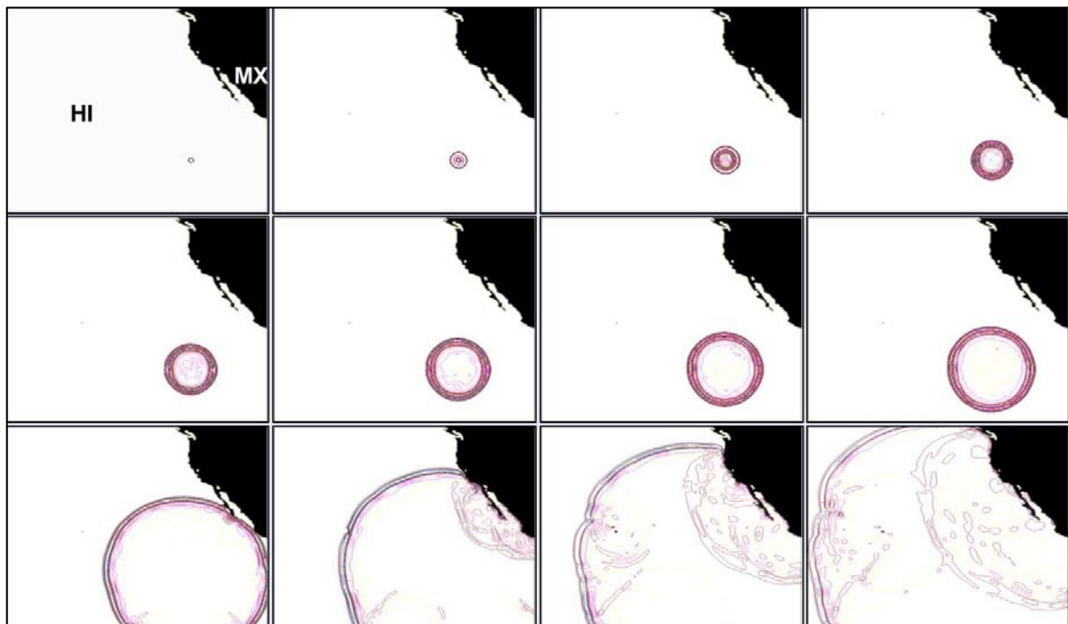
Figure 7: PDC 2015 TTX1: twelve snapshots of the numerical simulation of the ocean waves generation and propagation due to asteroid impact. Time flows from left to right and top to bottom.
