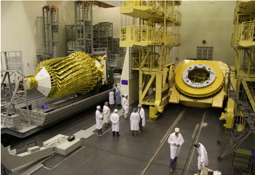
Figure 12: Spektr-R (RadioAstron) space-borne 10 m diameter radio telescope, undeployed (RIA Novosti archive, image #930415 / Oleg Urusov / CC-BY-SA 3.0)
