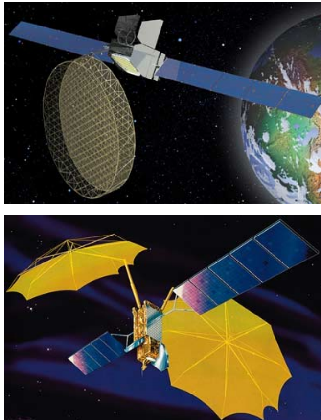
Figure 11: Large deployable antenna main reflectors on geosynchronous communication satellites for direct-to-satellite mobile phone systems - (top) Thuraya 2 and 3 design, 12.25 m antenna diameter (artists concept: Boeing BSS via Gunter's Space Page) - (top) Garuda-1 (ACeS-1) design, two times 12 m antenna diameter (Lockheed-Martin via Gunter's Space Page)
