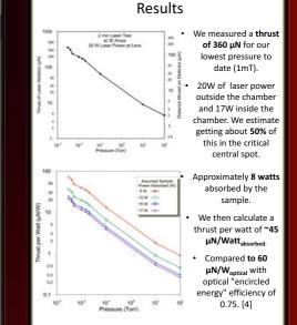
Our measurements of thrust become a lower limit to what will be encountered in a real target. Thus our measurements are extremely conservative compared to what can be achieved in an optimized system.
