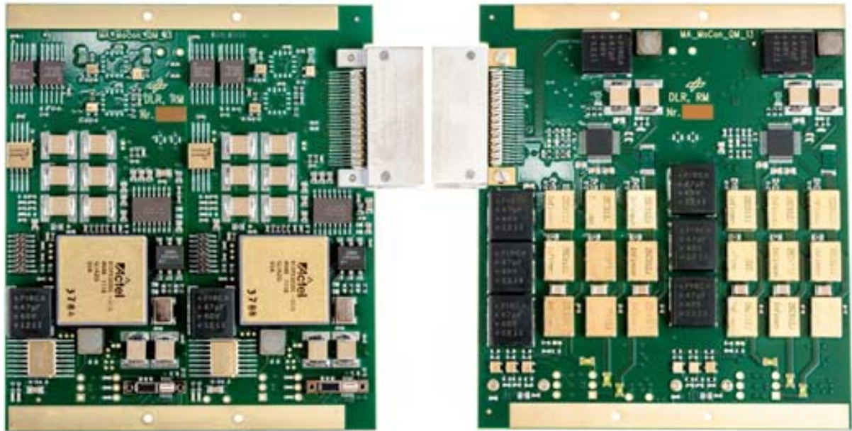
Figure 16: FM of MobCon motion controller PCB (left: top side, right: bottom side).
