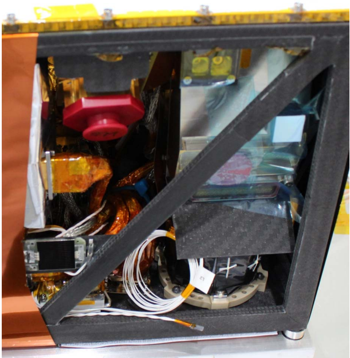
Figure 6 - Magnetometer FM integrated in the MASCOT, sensor crouching under camera in the lower right corner
