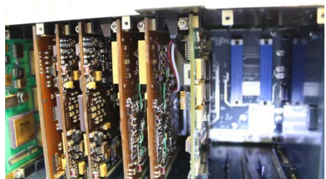
Figure II-2: View into MASCOT E-box with subsystem PCBs and instruments backend-electronics partially integrated
