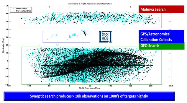
Figure 1. A Single Night's Worth of Resident Space Object (RSO Detections (for various orbital regions) from the U.S. Space Surveillance Telescope (SST) in New Mexico.
