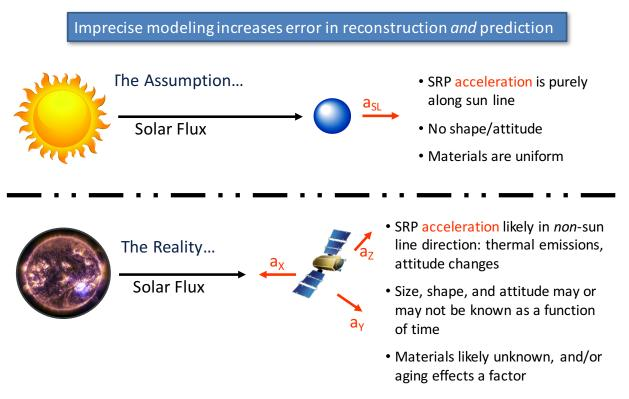
Figure 2. Difference between the motion experienced by a spherical (cannonball-like) space object and a satellite with realistic size, shape, orientation, and material properties. For the sphere, the acceleration due to the sun's effects are unidirectional. In reality, our tracking data informs us that objects experience accelerations due to the Sun's effects in 3dimensional space (multi-directional).
