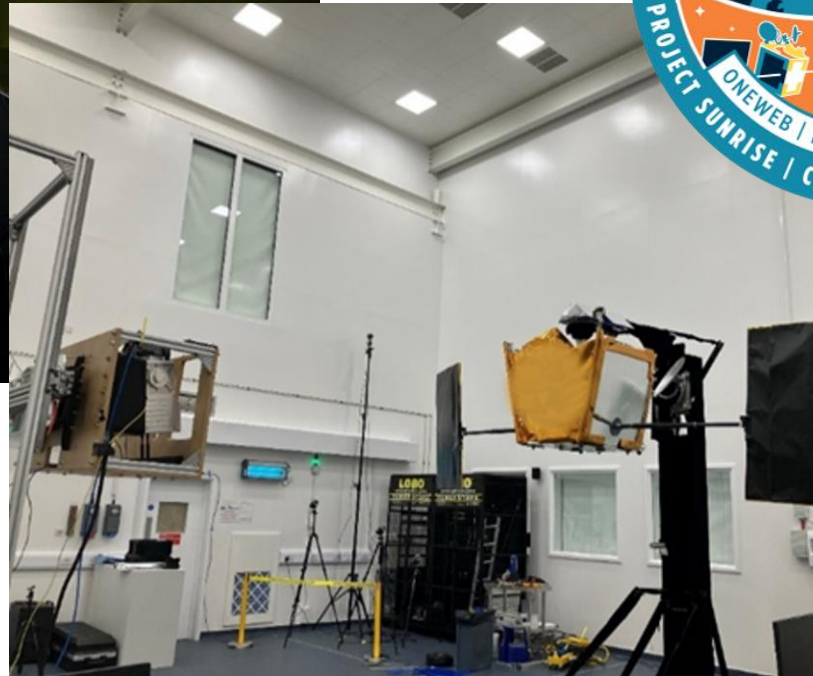
ELSA-M system and subsystems testing with OneWeb Gen 1 Mock-up
