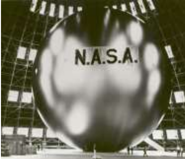
Figure 5.5 Echo II undergoing stress test (image credit NASA)
