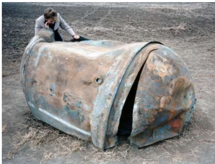
Figure 4.6 This Delta II Second Stage propellant tank survived re-entry. (Photo: NASA, https://orbitaldebris.jsc.nasa.gov/reentry/ , 6 March 2018)
