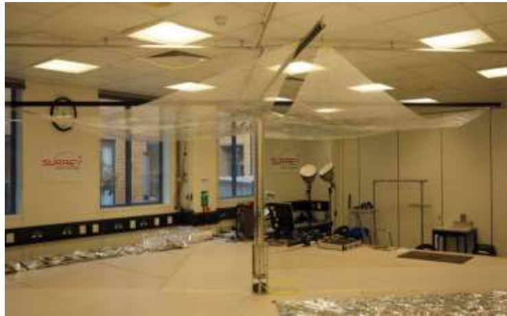
Figure 5.21 Surrey Space Centre's InflateSail: carbon-fibre boom tips are suspended from sliding gantry. (Image Credit: Surrey Space Center)
